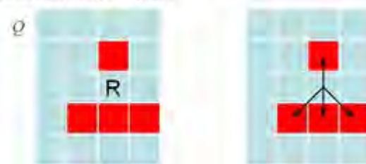
Figure 6: 180^\circ rotated edge points of Q around R (left) and four vectors of Q (right)
