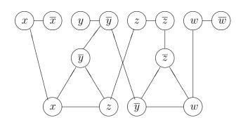
That finishes the description of G. Suppose that  $\phi$  has v variables and c clauses. Any vertex cover of G will need to have size at least v + 2c, one to cover each vertex gadget and two to cover each clause gadget. Let's choose k = v + 2c, not leaving any room for extra vertices in the vertex cover.
