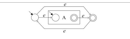
**Figure 8.4.** The regular languages are closed under Kleene closure. Suppose that A is a regular language. Get an NFA<sub> $\varepsilon$ </sub> for A, and assume that it has exactly one accepting state. Build an NFA<sub> $\varepsilon$ </sub> for A<sup>\*</sup> as shown in the diagram above.
