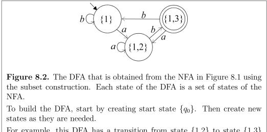
For example, this DFA has a transition from state  $\{1,2\}$  to state  $\{1,3\}$  labeled b because there is a transition in the DFA from 1 to 1 labeled b and there is also a transition from 2 to 3 labeled b.
