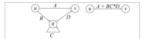
**Figure 8.5.** Choose a state q to remove that is not the start state and not the accepting state. First modify the transitions between states uand v for all pairs of states (u, v) where  $u \neq q$  and  $v \neq q$ . The left-hand diagram shows transitions from u to q, q to itself and q to v. The righthand diagram shows the new transition from u to v. Notice that the new regular expression labeling the transition from u to v makes it unnecessary to go through q.
