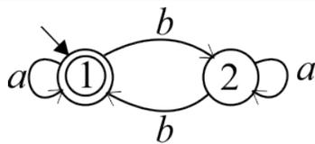
**Figure 5-1.** Transition diagram of FSM  $M_1$  that recognizes language  $\{s \in \{a, b\}^* \mid s \text{ has an even number of } a\text{'s}\}$ . There are two states. State 1 is the start state. State 1 is an accepting state and state 2 is a rejecting state..
