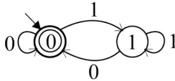
**Figure 5-4.** A FSM that recognizes even binary numbers. An empty string is treated as 0.
